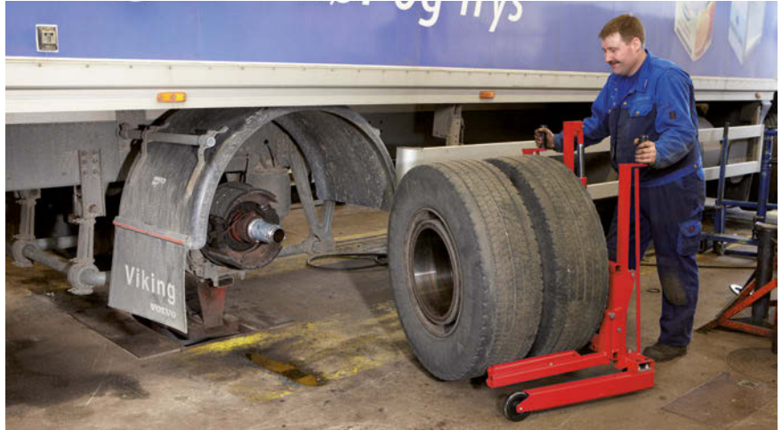
A high-lift wheel dolly allows wheel removal without back strain.
