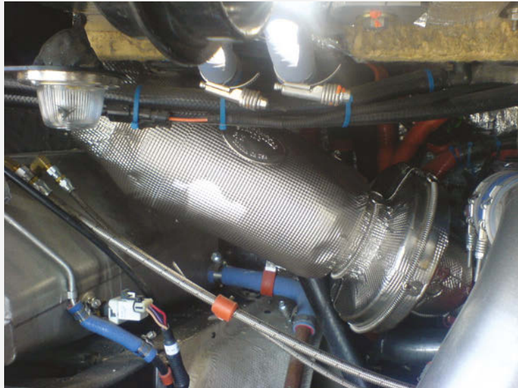
A view of a metal foil insulation blanket over an exhaust bellow within an engine compartment.
