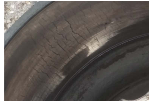
Pictured here is a worn brake drum.
