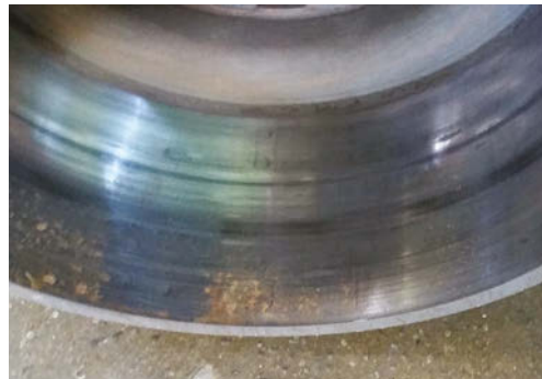
This drum, with less than 30,000 miles, shows early wear from aggressive friction material.
