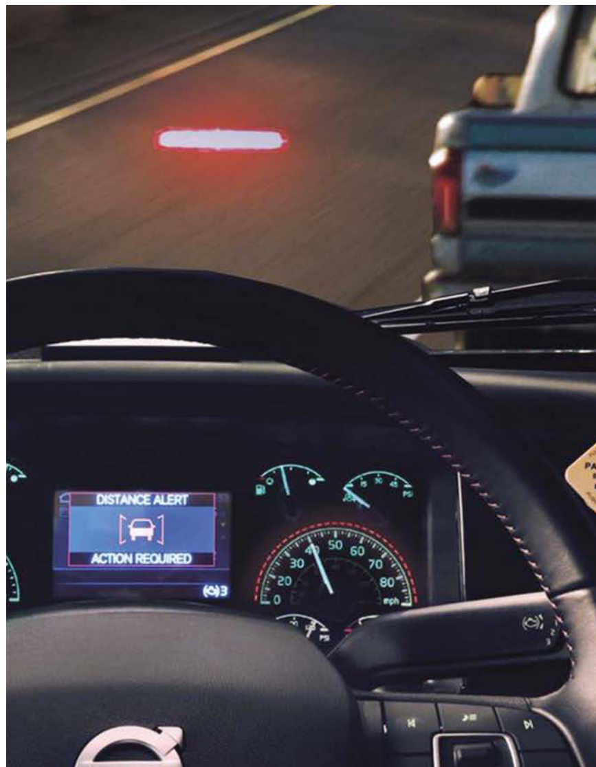
» Drivers are given visual and audible warnings when the system detects an impending collision.
