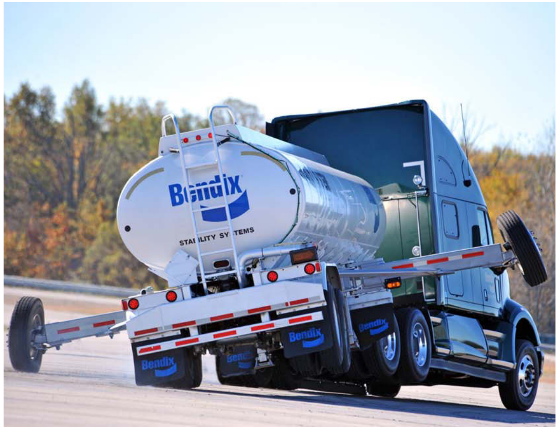
» A truck, shown on a demonstration track, with its electronic stability control system turned off (above) and on (below).
