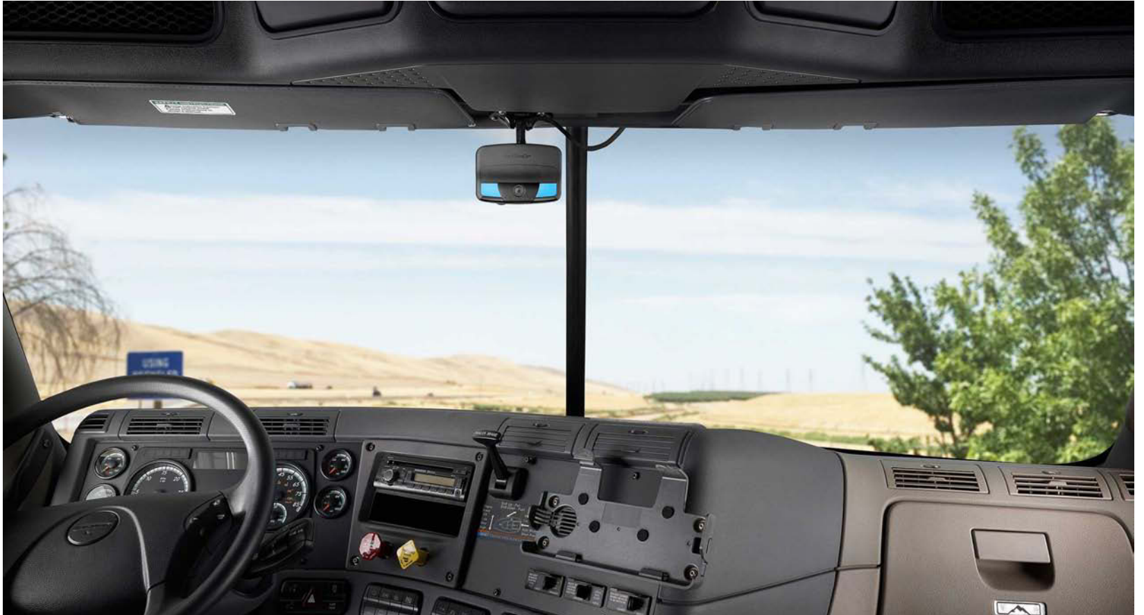
» Forward monitoring and driver monitoring cameras (above and right) mounted inside the cab.
