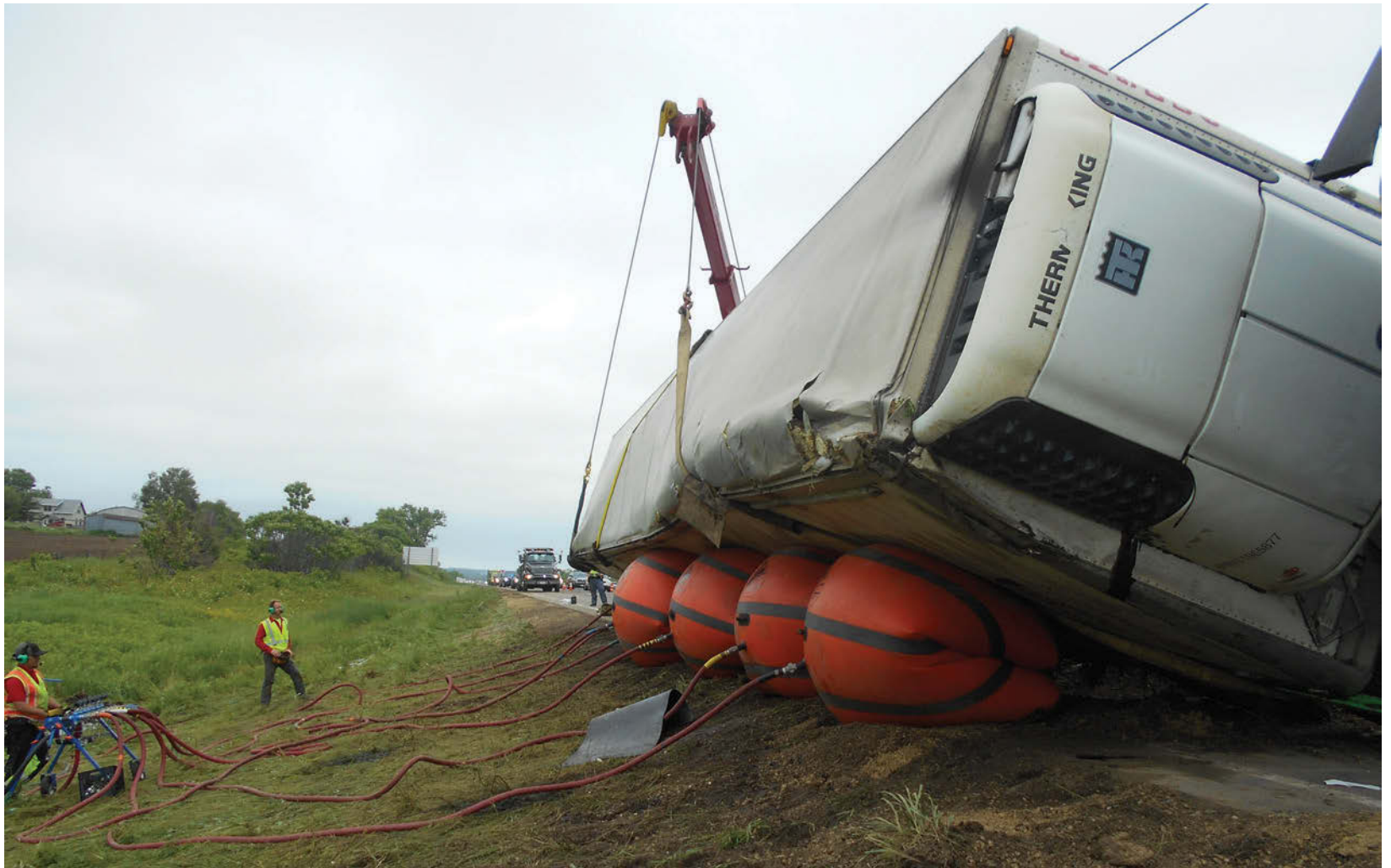
» Recovery air cushions are needed to upright a reefer loaded with produce to help maintain the structural integrity of the trailer.
