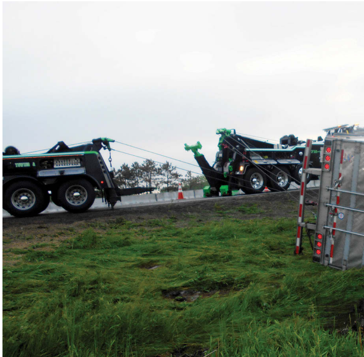
» Multiple heavy wreckers may be needed on-scene lifting together, depending on the recovery scenario, especially with a fully loaded trailer.
