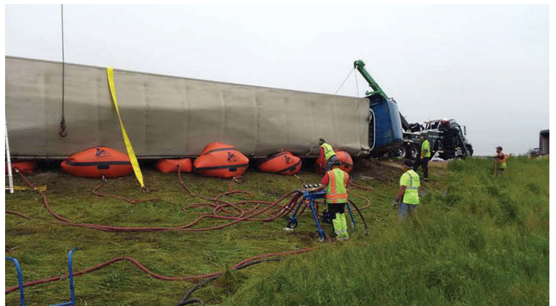
» The recovery cushions do not lift the compromised trailer alone but assist the heavy duty wrecker (or wreckers) on-scene with a safer lift.
