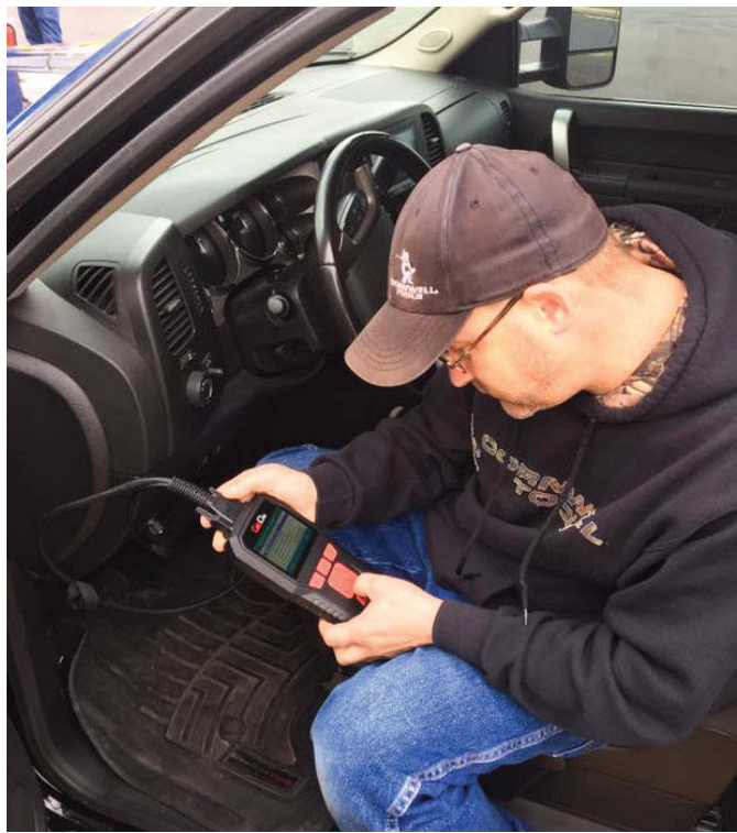
» Look for patterns of fault codes at certain mileage intervals, as they could indicate potential failures in the future.
