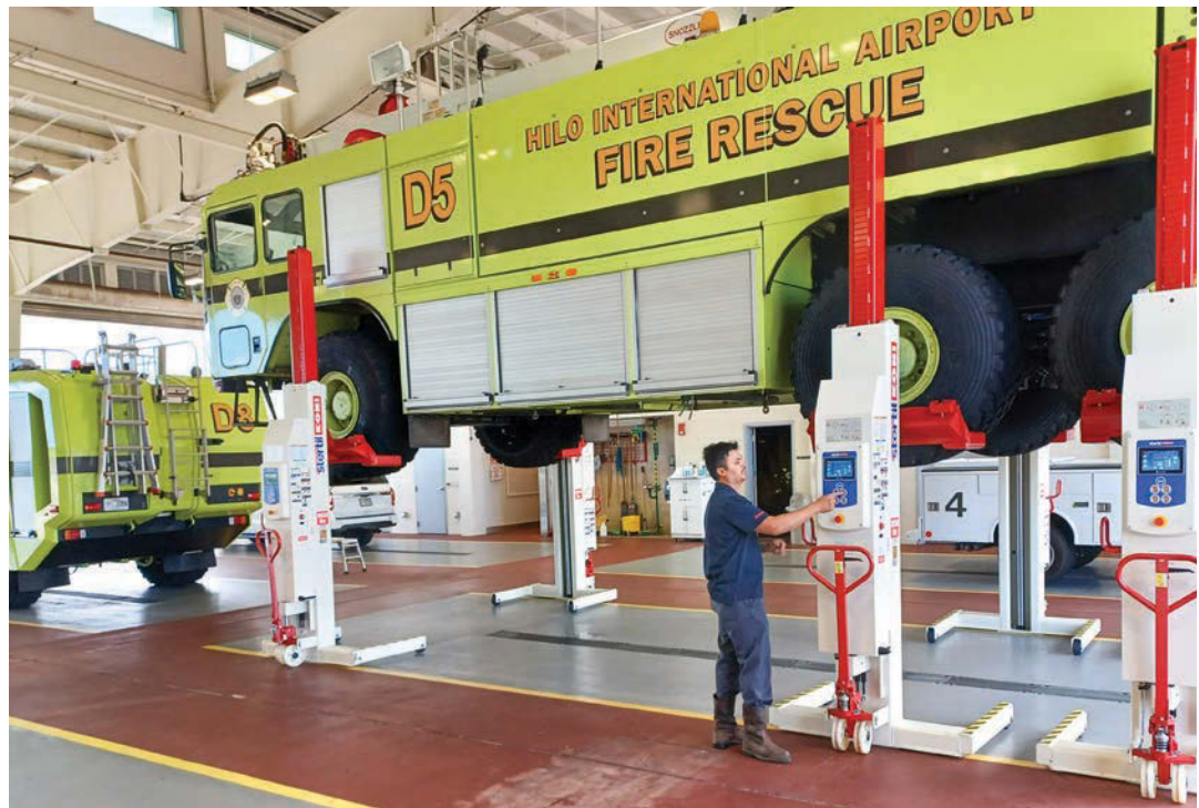
» The maintenance department at the State of Hawaii Airport Fire Department prefers mobile column lifts, as they can be configured for each type of vehicle in the fleet and at various service bays.
