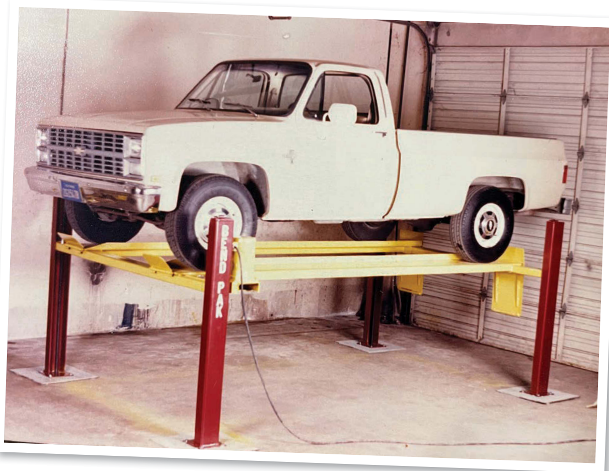
» BendPak's first car lift, circa 1983. It was a fully mechanical lift with chains, sprockets, and a single large electric motor for the drive system. After selling about 200, the company discontinued this model in favor of simpler hydraulic/chain-driven designs.
