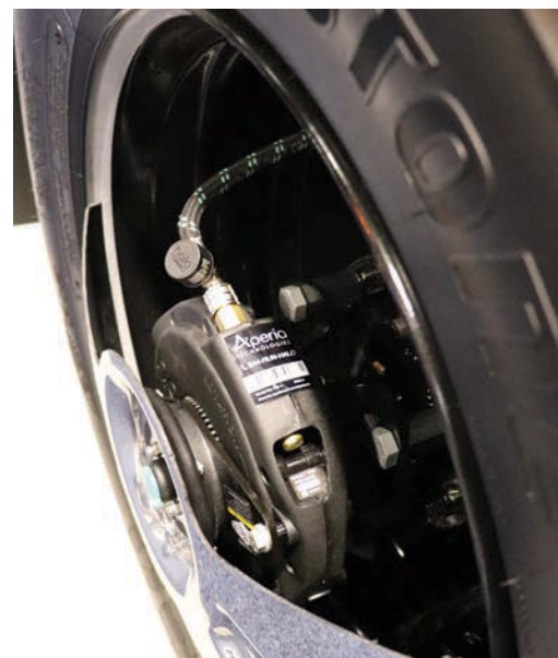
» Aperia’s Halo tire inflation system charges itself back up as the tire rolls.
