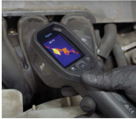
» Thermal imagery can provide a ‘before and after’ to verify completed repairs and ensure components are operating to specification.
