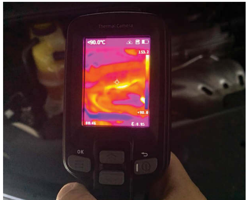
» Thermal imaging can validate vehicle temperature sensors and readings.
