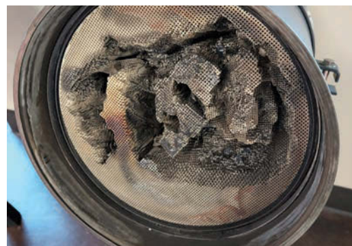
» Exothermal damage caused by over fueling or a high temperature condition.
