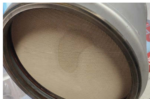
» Staining on an uncatyzed filter like this is not harmful if the cause was corrected.
