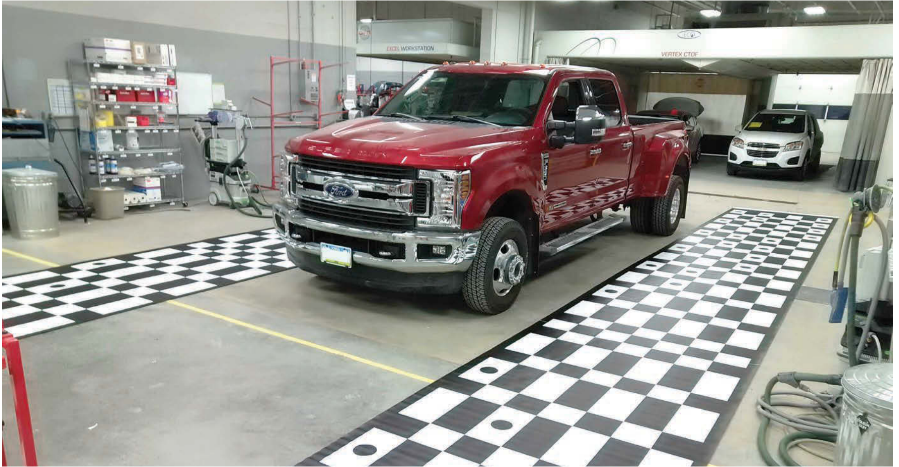
» Specific equipment is needed to perform static ADAS calibrations.
