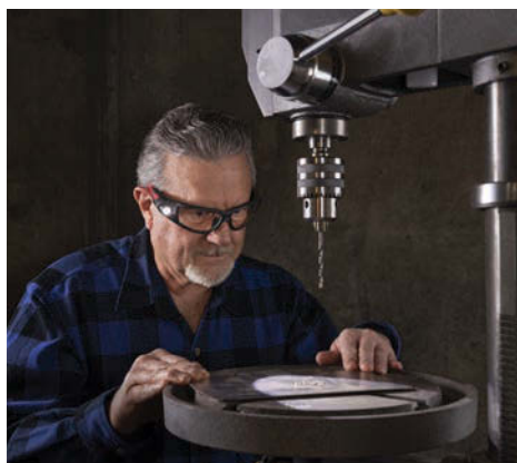
» Safety gear should be certified by ANSI. This is especially important for gear such as safety glasses, hard hats, and protective gloves to ensure they are manufactured to high enough standards to protect technicians from cuts, abrasions, and impacts.
