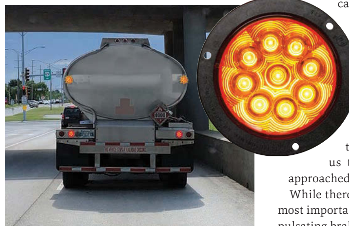
» Some fleets opt to use dual outboard lights. Mounting on a tank requires adhesive or brackets to avoid drilling or welding.
