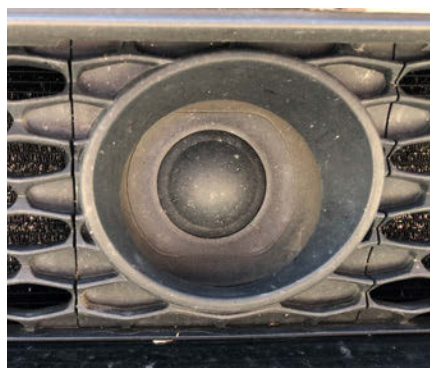
A dynamic calibration is performed (road test with scan tool) to teach the sensor to adapt and function properly. This is Chrysler Pacifica’s ACC radar sensor.
