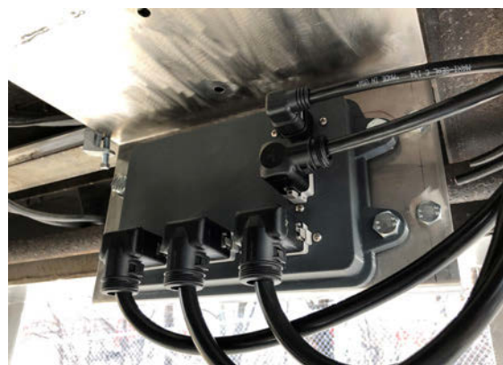
Mitigating electrical issues by periodically check all connections and plugs on a fleet's vehicles and replace them with newer, more weather- and corrosion-resistant components.
