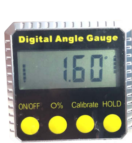
A static calibration can also be completed more easily with a modern digital angle gauge. Turn a screw and adjust the ACC radar module’s vertical aim.
