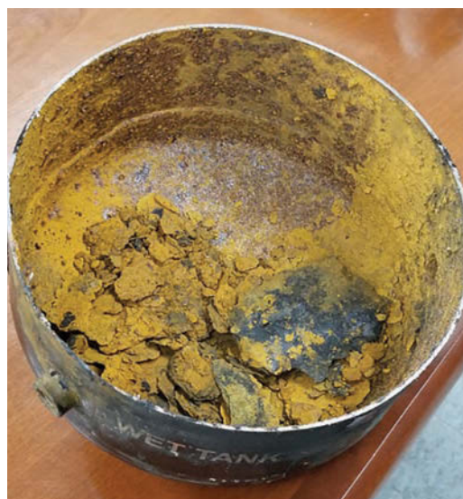
» Contaminant build-up in pneumatic systems leads to premature component wear and tear.
