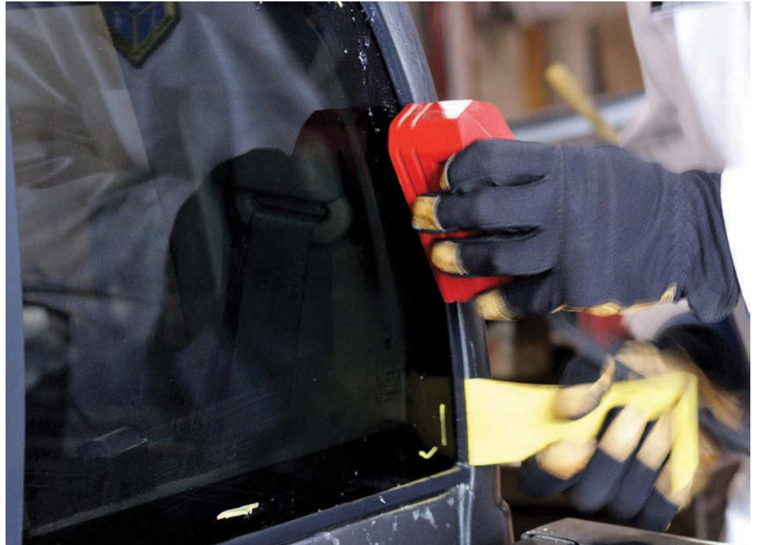
» Inductor Glass Blasters help technicians safely remove damaged windshields for replacement.
