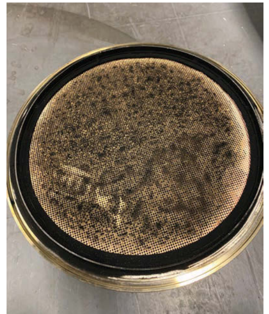
» Example of a failed DPF caused by excessive soot buildup over time. When servicing older vehicles in particular, a technician should look for obvious signs of soot bypass (as shown) to know the DPF has failed and should be replaced. This is also a good time to consider replacing the DOC.
