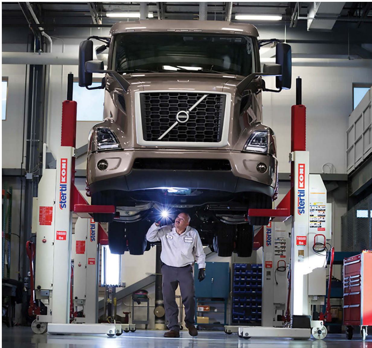
» A technician inspects the underbody of a vehicle using a four-post lift, a key component to shop safety. Stertil-Koni
